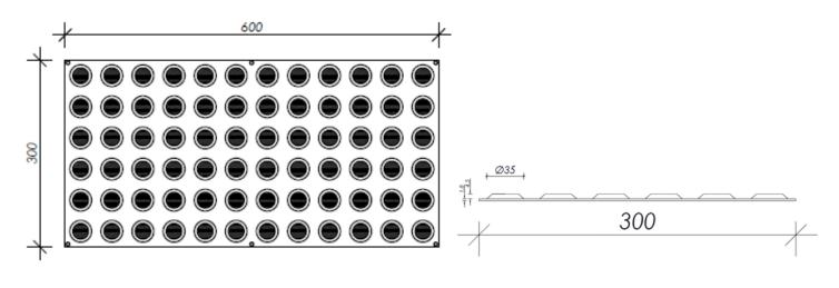
**FIXING** Drill or Diamond core & fix with Screw and Poly-anchor
