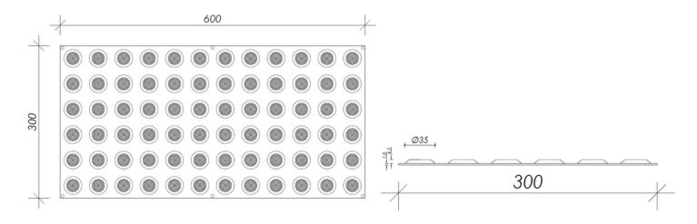
**FIXING** Drill or Diamond core & fix with Screw and Poly-anchor
