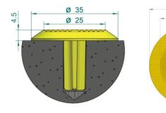
**FIXING** Core Drill and Pressure Fitted
