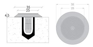
**FIXING** Core Drill and Pressure Fitted
