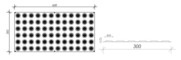
**FIXING** Drill or Diamond core & fix with Screw and Poly-anchor
